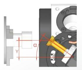
The workpiece axis and the skiving tool axis must be related to each other in a defined angle ( $\alpha).$
