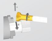
When skiving is finished the cutter has to move towards X.
