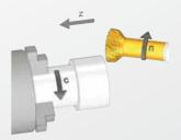
Synchronization of work piece and tool rotation.
